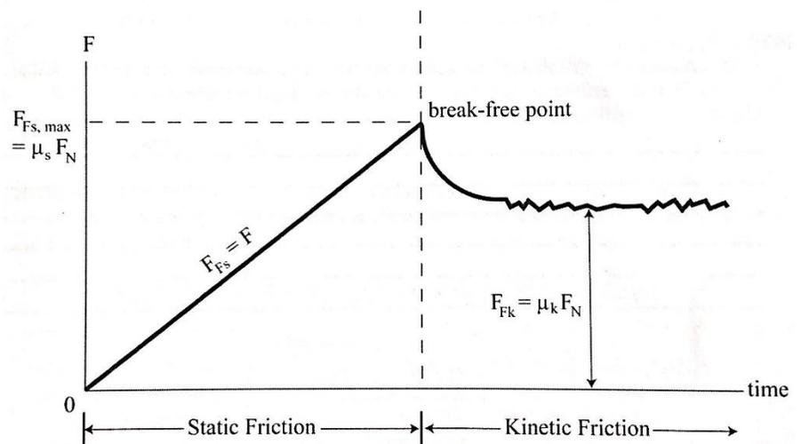
**Part 1: Measuring the Coefficient of Friction:** *In this part of the lab you will measure the coefficient of friction (both static and kinetic) between a block of wood and an aluminum surface, or another surface of your choice. You will also vary the normal force on the block by incrementally increasing the mass.*
