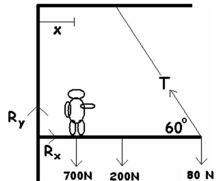
**Q14:** Examine the diagram of a bear on a pole. The string (T) can hold a total of 900 N. Can the bear reach the 80-N basket of food without the string breaking? The total distance out to the food is 6-m.
