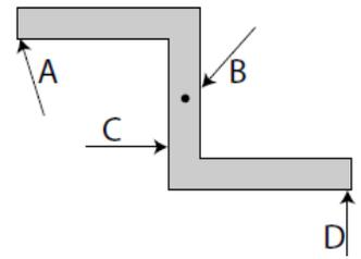
**Q6.** A constant force  $F$  is applied for five seconds at various points of the object, as shown in the diagram. Rank the magnitude of the torque exerted by the force on the object about an axle located at the center of mass from smallest to largest.
