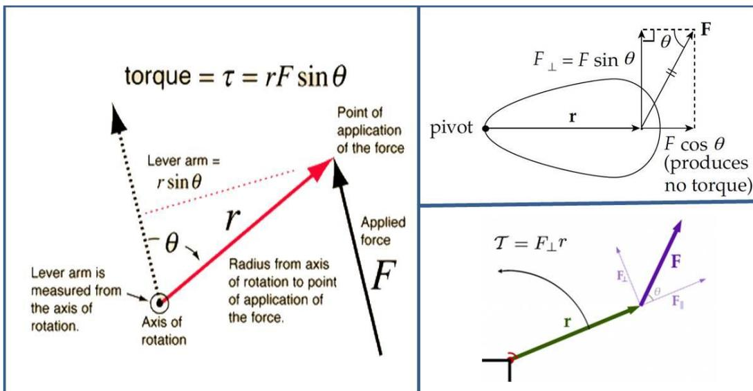
**Q4:** A captain of a ship turns the stirring wheel by applying a 20 N torque. If he applies the force at a radius of 0.2 m from the axis of rotation, at an angle of 80 degrees to the line of action (moment arm), what torque does he apply?
