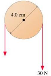
**Q7.** A student pulls down on a small modified Atwood machine with a force of 30 N, as shown in the diagram. What is the torque of this force?
