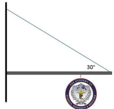
**FACT:** In table/bridge problems the fulcrum (pivot point) is arbitrary because the object is not rotating. Choose one of the supports as the fulcrum, which means that point now has zero torque ( $r = 0$ ).
