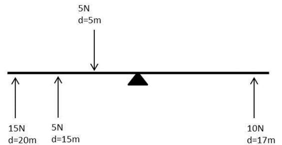
**Q9.** Forces are applied along various points on a lever arm as shown. Calculate the net torque and describe the resulting motion of the lever. Determine the force and distance from the axis of rotation that would result in a net moment (torque) of zero.
