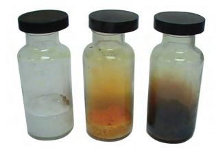
Figure 18.60 Chlorine is a pale yellow-green gas (left), gaseous bromine is deep orange (center), and gaseous iodine is purple (right). (Fluorine is so reactive that it is too dangerous to handle.) (credit: Sahar Atwa)
