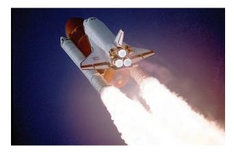
Figure 18.28 Before the fleet's retirement in 2011, liquid hydrogen and liquid oxygen were used in the three main engines of a space shuttle. Two compartments in the large tank held these liquids until the shuttle was launched. (credit: "reynermedia"/Flickr)
