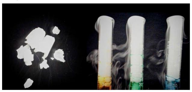
Figure 10.1 Solid carbon dioxide ("dry ice", left) sublimes vigorously when placed in a liquid (right), cooling the liquid and generating a fog of condensed water vapor above the cylinder. (credit: modification of work by Paul Flowers)
