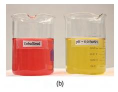
Figure 14.17 (a) The buffered solution on the left and the unbuffered solution on the right have the same pH (pH 8); they are basic, showing the yellow color of the indicator methyl orange at this pH. (b) After the addition of 1 mL of a 0.01-*M* HCl solution, the buffered solution has not detectably changed its pH but the unbuffered solution has become acidic, as indicated by the change in color of the methyl orange, which turns red at a pH of about 4. (credit: modification of work by Mark Ott)
