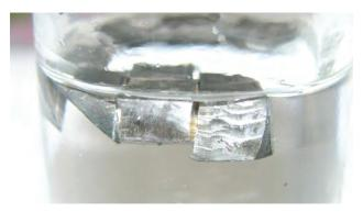
Figure 18.3 Lithium floats in paraffin oil because its density is less than the density of paraffin oil.
