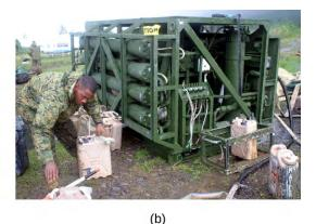
Figure 11.27 Reverse osmosis systems for purifying drinking water are shown here on (a) small and (b) large scales. (credit a: modification of work by Jerry Kirkhart; credit b: modification of work by Willard J. Lathrop)
