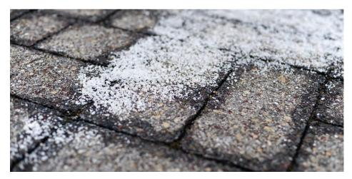
Figure 11.22 Rock salt (NaCl), calcium chloride (CaCl<sub>2</sub>), or a mixture of the two are used to melt ice. (credit: modification of work by Eddie Welker)
