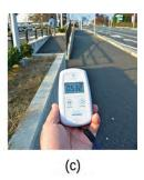
Figure 21.35 Devices such as (a) Geiger counters, (b) scintillators, and (c) dosimeters can be used to measure radiation. (credit c: modification of work by "osaMu"/Wikimedia commons)
