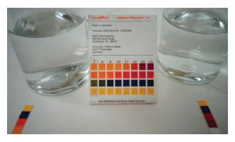
Figure 14.10 pH paper indicates that a 0.1-M solution of NH<sub>3</sub> (left) is weakly basic. The solution has a pOH of 3 ([OH<sup>-</sup>] = 0.001 M) because the weak base NH<sub>3</sub> only partially reacts with water. A 0.1-M solution of NaOH (right) has a pOH of 1 because NaOH is a strong base. (credit: modification of work by Sahar Atwa)
