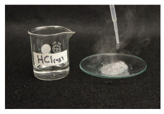
Figure 18.27 The reaction of iron with an acid produces hydrogen. Here, iron reacts with hydrochloric acid. (credit: Mark Ott)
