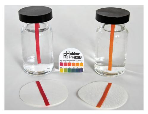
Figure 14.9 pH paper indicates that a 0.I-M solution of HCI (beaker on left) has a pH of 1. The acid is fully ionized and  $[H_3O^+]=0.1~M$ . A 0.1-M solution of CH<sub>3</sub>CO<sub>2</sub>H (beaker on right) is has a pH of 3 ( $[H_3O^+]=0.001~M$ ) because the weak acid CH<sub>3</sub>CO<sub>2</sub>H is only partially ionized. In this solution,  $[H_3O^+]<[CH_3CO_2H]$ . (credit: modification of work by Sahar Atwa)
