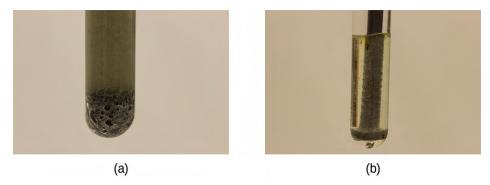
Figure 12.6 (a) Iron powder reacts rapidly with dilute hydrochloric acid and produces bubbles of hydrogen gas because the powder has a large total surface area:  $2Fe(s) + 6HCl(aq) \longrightarrow 2FeCl3(aq) + 3H2(g)$ . (b) An iron nail reacts more slowly.
