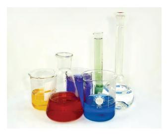
**Figure 18.15** Laboratory glassware, such as Pyrex and Kimax, is made of borosilicate glass because it does not break when heated. The inclusion of borates in the glass helps to mediate the effects of thermal expansion and contraction. This reduces the likelihood of thermal shock, which causes silicate glass to crack upon rapid heating or cooling. (credit: "Tweenk"/Wikimedia Commons)
