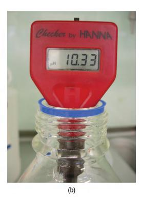
**Figure 14.4** (a) A research-grade pH meter used in a laboratory can have a resolution of 0.001 pH units, an accuracy of ± 0.002 pH units, and may cost in excess of \$1000. (b) A portable pH meter has lower resolution (0.01 pH units), lower accuracy (± 0.2 pH units), and a far lower price tag. (credit b: modification of work by Jacopo Werther)
