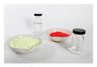
Figure 3.6 Each sample contains  $6.02 \times 10^{23}$  molecules or formula units—1.00 mol of the compound or element. Clock-wise from the upper left: 130.2 g of C<sub>8</sub>H<sub>17</sub>OH (1-octanol, formula mass 130.2 amu), 454.9 g of Hgl<sub>2</sub> (mercury(II) iodide, formula mass 459.9 amu), 32.0 g of CH<sub>3</sub>OH (methanol, formula mass 32.0 amu) and 256.5 g of S<sub>8</sub> (sulfur, formula mass 256.6 amu). (credit: Sahar Atwa)
