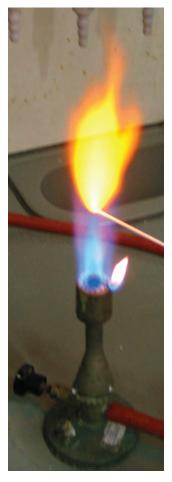
Figure 18.5 Dipping a wire into a solution of a sodium salt and then heating the wire causes emission of a bright yellow light, characteristic of sodium.
