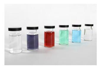
**Figure 19.12** Metal ions that contain partially filled d subshell usually form colored complex ions; ions with empty d subshell ( $d^0$ ) or with filled d subshells ( $d^{10}$ ) usually form colorless complexes. This figure shows, from left to right, solutions containing  $[M(H_2O)_6]^{n+}$  ions with  $M = Sc^{3+}(d^0)$ ,  $Cr^{3+}(d^3)$ ,  $Co^{2+}(d^7)$ ,  $Ni^{2+}(d^8)$ ,  $Cu^{2+}(d^9)$ , and  $Zn^{2+}(d^{10})$ . (credit: Sahar Atwa)
