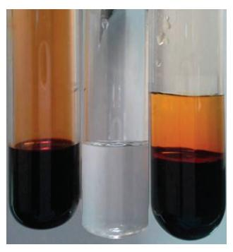
Figure 11.16 Bromine (the deep orange liquid on the left) and water (the clear liquid in the middle) are partially miscible. The top layer in the mixture on the right is a saturated solution of bromine in water; the bottom layer is a saturated solution of water in bromine. (credit: Paul Flowers)
