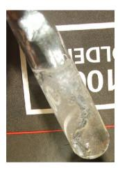
**Figure 18.7** Zinc is an active transition metal. It dissolves in hydrochloric acid, forming a solution of colorless Zn<sup>2+</sup> ions, Cl<sup>-</sup> ions, and hydrogen gas.
