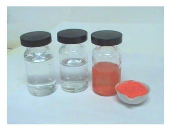
Figure 18.61 Solid HgI2 forms when solutions of KI and Hg(NO<sub>3</sub>)<sub>2</sub> are mixed. (credit: Sahar Atwa)
