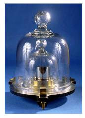
Figure 1.24 This replica prototype kilogram is housed at the National Institute of Standards and Technology (NIST) in Maryland. (credit: National Institutes of Standards and Technology)
