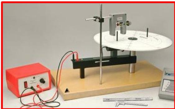
**Figure 1:** The rotational apparatus set-up with the power supply at 3 volts and the photogate positioned so it will not hit the pegs as it rotates. Calipers may be needed depending on your experimental design. Please turn off the power supply when it is not in use to ensure the fuse does not blow.
