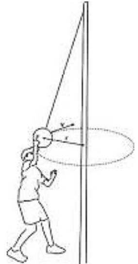
*A tetherball behaves similar to a conical pendulum, in that the x-component of the tension of the rope provides the centripetal force needed to keep the ball traveling in a circle while the y-component of the tension counters the weight of the ball.*
